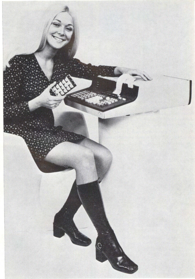
NEW GENERATION. Hewlett-Packard's new Series 9800 Model 10 programmable calculator has six times' memory capacity of comparably priced units, and is first to use plug-in function blocks (about the size of a deck of cards) to expand operational capabilities. Model 10 has wide range of optional accessories to enable user to tailor unit to his specific needs. Basic calculator, which sells for $2,975, has 51 registers and 500 program steps. As a teaching aid, the 9800 Model 10 is designed for broad application in mathematical, engineering, and scientific education and related fields.
